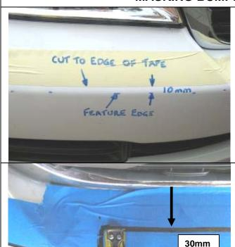
Apply wide masking tape edge, carefully aligning 10mm above bumper feature line as shown. Keep the same line level through the centre section of the bumper as shown
