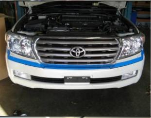
12. Apply approx.200mm of masking tape with edge exactly 90mm from angled bumper end as shown.
