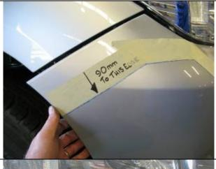
19. Pull outer returns of bumper outwards and out of retaining clips.
