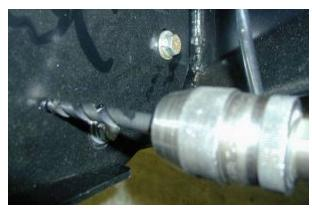
73. Using the M10 pilot holes in mount brackets (located up 175mm from bottom face of bar), drill pinning hole through uprights on bull bar. Fit M10 screw, washer set and flange nut and do up tight.
