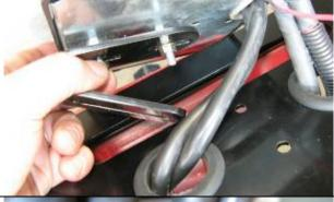
44. Fit control box bracket to control box studs as shown. *Picture also shows routing of leads through grommets in pan.*
