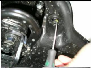
When removing lower trim panels, a plastic nut located on each side will need to be prized open with a small flat blade screwdriver to assist removal.
