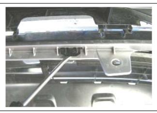
24. Remove grille from bumper cover by releasing plastic tabs as shown
