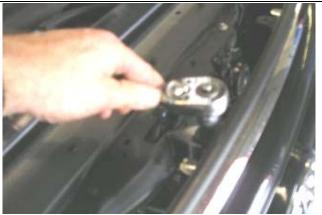
8. Remove retaining screws from top of grille
