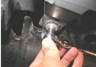
6. Remove lower bumper retaining screws.
