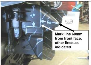
32. Mark the lower section of the air scoop for the power steering radiator as shown. This is for trimming to clear the mount brackets.
