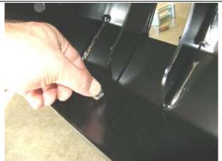
58. Fit 4 x M6 cage nuts to bottom inside face of lower pan in square holes as shown.
