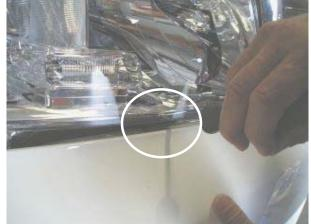
20. Push bumper down immediately below headlamp to gain access with a small flat blade screwdriver and release holding tab.
